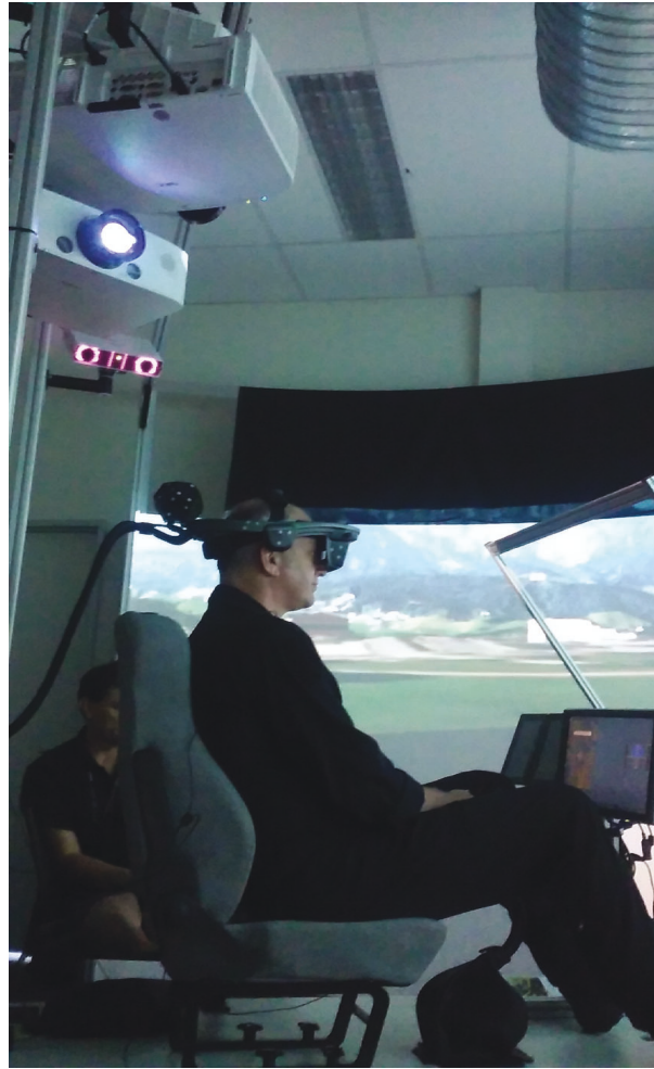
FIGURE A.1: An example of the simulator setup. The pilot has the head piece attached which displays the HUD information over the simulated environment. In front of the pilot are the electronic map and a multi-function display, which indicated altitude, ground speed, collective power and helicopter roll.
